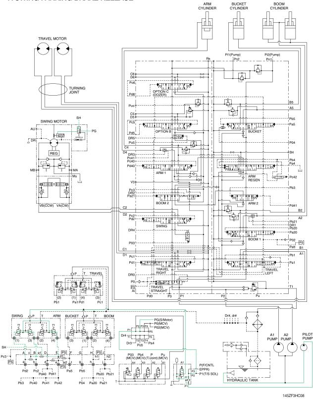
When any one of the swing, arm in, boom up or travel lever is tilted, the swing brake solenoid valve is shifted to the downward by the MCU that senses the pilot pressure of the RCV control lever.
