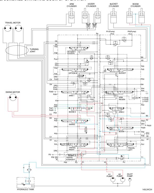
When the swing and boom up functions are operated simultaneously, the swing spool and boom spools in the main control valve are moved to the functional position by the pilot oil pressure (Pc2, Pd2, Pa20, Pa21) from the remote control valve.
