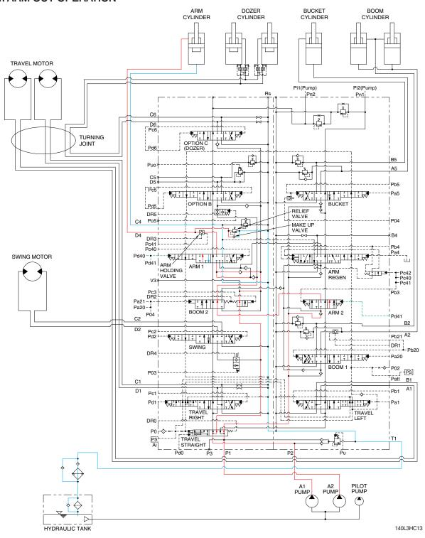
When the left control lever is pushed forward, the arm spools in the main control valve are moved to the arm out position by the pilot oil pressure (Pd40, Pd41) from the remote control valve.
