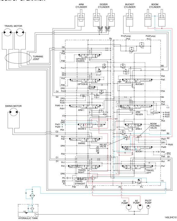
When the right control lever is pulled back, the boom spools in the main control valve are moved to the up position by the pilot oil pressure (Pa20, Pa21) from the remote control valve.
