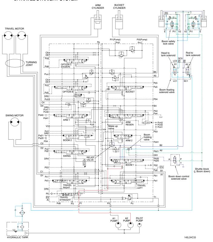
When the travel and other functions (boom, arm, bucket, swing, option) are tilted, the travel straight EPPR valve is energized by the MCU that senses the pilot pressure of the travel and other functions and Pd0 pressure from the travel straight EPPR valve changes the travel straight spool.
