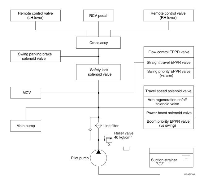
The pilot circuit consists of suction circuit, delivery circuit and return circuit.
